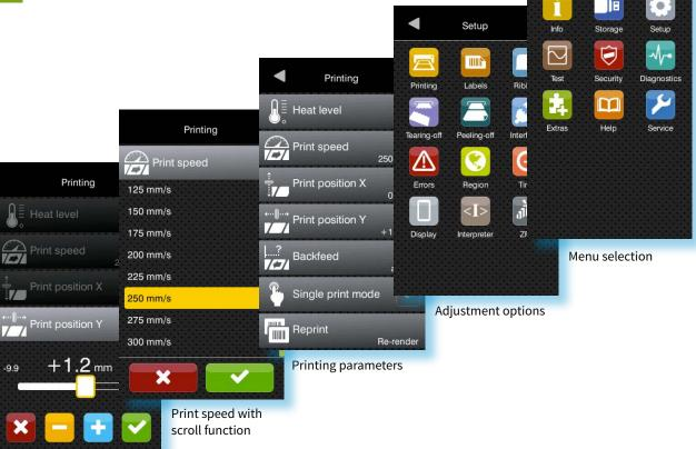
Printing offset y slide control for fast adjustment +/- keys for fine adjustment
